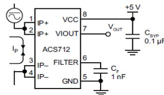
Application 1. The ACS712 outputs an analog signal,  $V_{OUT}$ , that varies linearly with the uni- or bi-directional AC or DC primary sampled current,  $I_p$ , within the range specified.  $C_F$  is recommended for noise management, with values that depend on the application.
